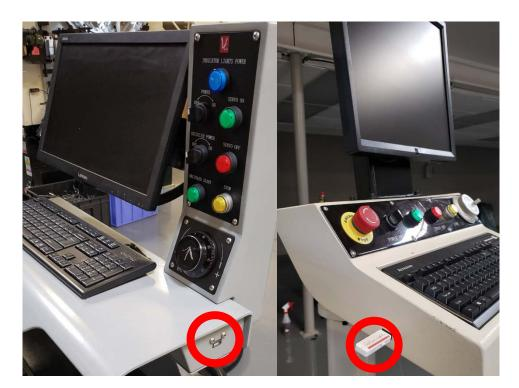
b. Start up the computer and when the follow screen is displayed, press the "Delete" key on the keyboard
