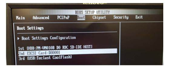
e. The bottom right corner will provide options. Select the drive you would like to switch. In this case, switch the [SCSI Card: xxxx] with the [HDD:xxx] order. Press "Enter" once you have selected the backup drive.
