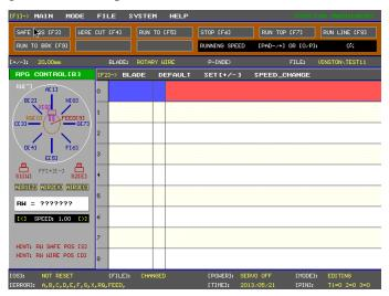
Step 3: On the top left hand corner of the figure below, you see [OS]: NOT RESET, which indicates that the system needs to reset itself. The bottom left hand corner ("[ERROR]") prompts for any error messages from each axis such as A, B, RQ, etc. The primary reason that the errors show up after start-up is the servo motors are not turned on.
