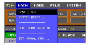
Press the ▼ arrow key twice until "SHUT DOWN (CTRL - Q)" is highlighted and press the ENTER key.
