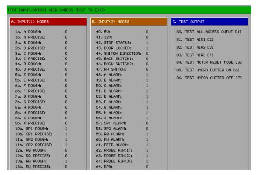
The list of inputs and outputs throughout the various regions of the machine are constantly tested while in this mode.
