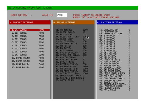
Press the ◀ ▶ arrows located on the keyboard. The user can return to the main program at any time by pressing the ESC key. Edit the value [>] of the current selection and press the INS (INSERT) key on your keyboard to save the changes.
