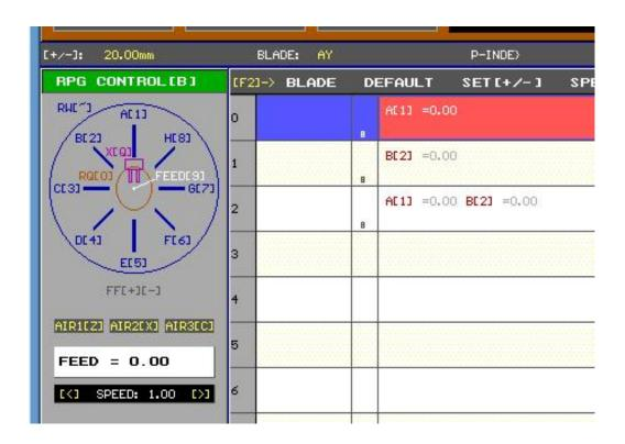
The RPG CONTROL window indicates the current position and the sensitivity of movements for the selected axis. The axis is moved manually and when the slide is in the correct position, it can be saved into the program as a save point. The operator will use the keys to select the programming line in the program to save the position of the slide. One the programming line has been selected, press the INS key to save the position of the axis. The following screen will appear:
