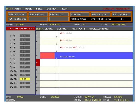
The user can also move the axis with the command RPG CONTROL. The sensitivity of the axis can be adjusted by using the "<" and ">" keys on the keyboard. The incremental movement of the axis can be adjusted to 0.01 mm, 0.50 mm, 1.00 mm, 2.00 mm and 4.00 mm. Use the INS (Insert) key to save the position of the axis. Repeat process for all axes that are listed in the current line of code.
