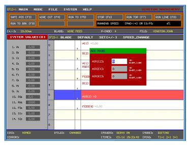
The pneumatic probe is enabled with a value of 1 and disabled with a value of 0. Whenever a pneumatic probe is enabled, it must be manually disabled within the program at a later point. It will not automatically retract after completing the designated task.
