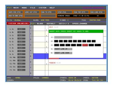
Highlight the AIR [Z] selection and press the INSERT key. With the Air [Z] component highlighted within the program line, press the ENTER key to configure the pneumatic probe:
