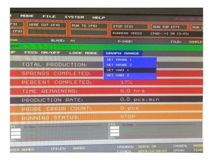
Press ENTER to bring up the selection window of the value for the variation tolerance of touch probe 1. The set value is 30%, meaning the feed viaration can be  $\pm$  30% of the default 10 mm feed.
