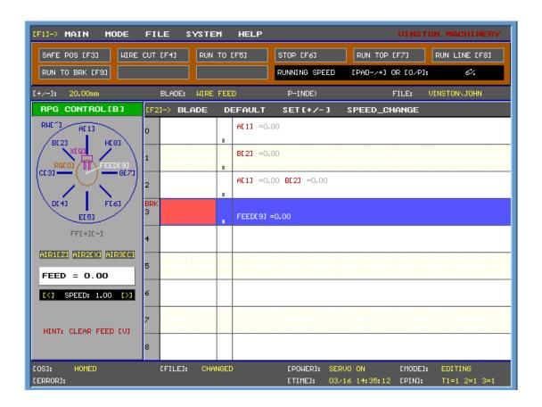
Using the three shortcut keys "Z", "X", "C" allows the user to manually turn the pneumatic cylinders on and off. Pressing each shortcut key once will change the current value from a 1 (Enabled) to a 0 (Disabled) or vise versa. This function is useful in the early stages of developing the program or to test the connections.
