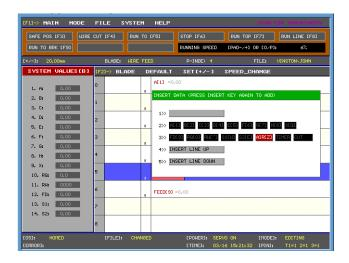
Select the AIR [Z] component and press the INSERT key. Set the AIR [Z] value back to 0 to retract the pneumatic probe.
