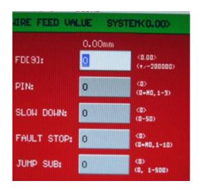
The first row, FD[9], allows the user to set the feed length of the wire before the probe comes into contact with the wire. The software will stop the wire feed once contact is made with the contact probe. If the wire does not come into contact with the probe, then the program can be configured to either move on to the next program line or stop and/or jump to a different section of the program.
