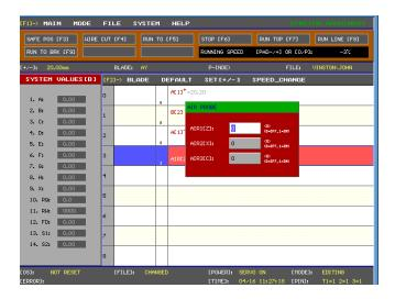
Set the value of the pneumatic cylinder in use to a value of 1.
