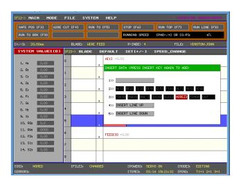
Select the AIR [Z] axis and press the Insert key.
