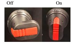
2) Turn the "POWER ON" knob located on the control panel clockwise to turn on the computer system and auxiliary circuits for the servo drivers.
