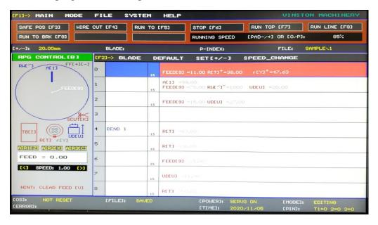
Step 3: On the top left hand corner of the figure below, you see [OS]: NOT RESET, which indicates that the system needs to reset itself. The bottom left hand corner ("[ERROR]") prompts for any error messages from each axis such as A, B, RQ, etc. The primary reason that the errors show up after start-up is the servo motors are not turned on.
