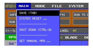
Press the ▼ arrow key twice until "SHUT DOWN (CTRL - Q)" is highlighted and press the ENTER key.
