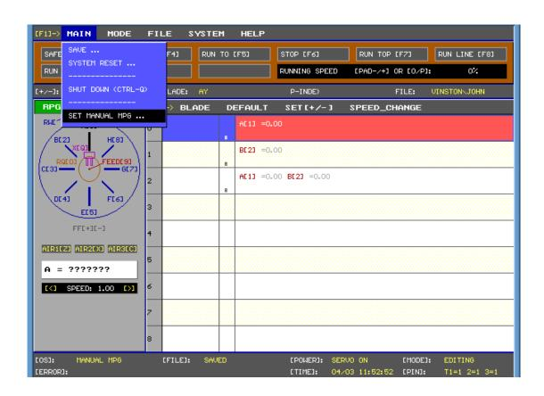
Select the axis to be moved. Use the numeric keys (the ones above the letters, not from the keypad) 1 thru 8 for the front slides, 9 for wire feed, 0 for the quill, ~ for RW (Rotating Wire) and Q for the X-Y blade. Movement of the selected axis is now controlled by the RPG dial on the control panel. When the axes have been adjusted, press the F3 key to return the machine back to EDIT mode.
