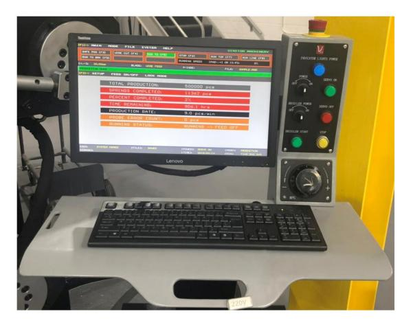
At this point, flip the machine power source to the OFF position. This switch works as the machines disconnect and all power is cut off from the machine.
