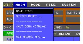
To perform a reset pressing the F1 key on the keyboard. Press the ▼ arrow once so that "SYSTEM RESET ..." is highlighted. Press the ENTER key on the keyboard (To exit out of the menu at any time, press the ESC key). The following message will appear after you select a system reset:
