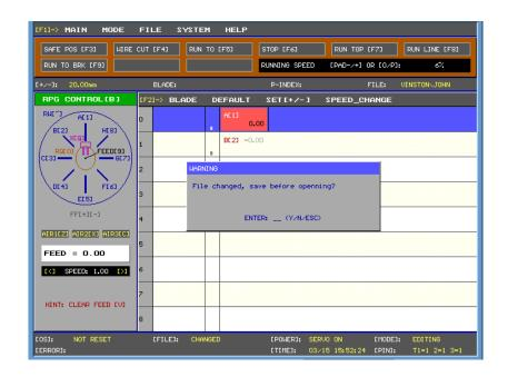
Press the Y key to save changes, the N key to continue without saving the current program or press ESC to cancel the selection. After pressing the Y, the user will be able to select a new program from a list of files.
