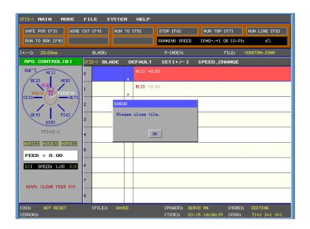
Confirm by pressing ENTER. After closing the current program and selecting to create a new program, the user will see the follow screen. After entering a file name, press the INS key to save the new program. Follow the same procedure for creating a folder instead of a file.
