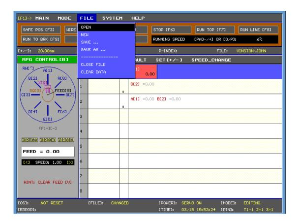
Press F1 to access the main menu bar. To navigate through the main menu, move the arrow keys  $\blacktriangleleft \triangleright$  located on the keyboard. To exit the main menu bar, press ESC.
