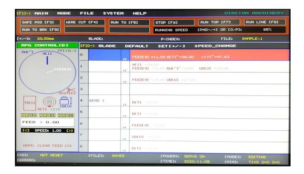
The selected axis can be moved by turning the RPG. Turning the RPG clockwise will correspond to a forward movement and turning it counterclockwise will correspond to a backward movement. Press "<" and ">" keys on they keyboard can be used to increase or decrease the sensitivity of the axis. The movement of the axis can be incrementally changed between 0.01 mm, 0.50 mm, 1.00 mm, 2.00 mm and 4.00 mm.
