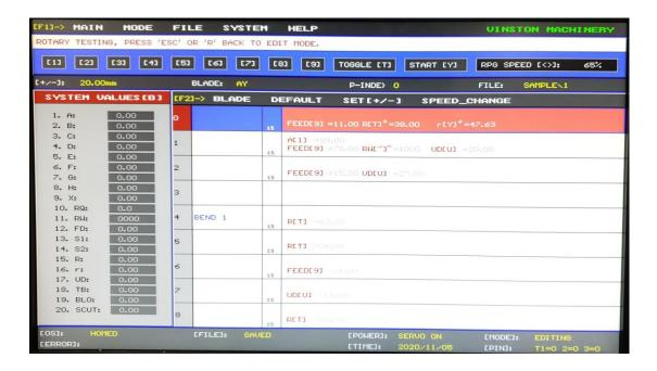
The left column indicates the current position of each axis. Rotating the RPG CONTROL will progressively move the active axis to the values indicated in the current highlighted line of code. The active axis will be highlighted in yellow while all other inactive axes will be in grey. The numeric keys 1 thru 9 can be used for incremental movements in place of
