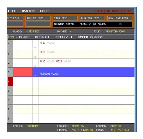
The user can also move the axis with the command RPG CONTROL. The sensitivity of the axis can be adjusted by using the "<" and ">" keys on the keyboard. The incremental movement of the axis can be adjusted to 0.01 mm, 0.50 mm, 1.00 mm, 2.00 mm and 4.00 mm. Use the INS (Insert) key to save the position of the axis. Repeat process for all axes that are listed in the current line of code.
