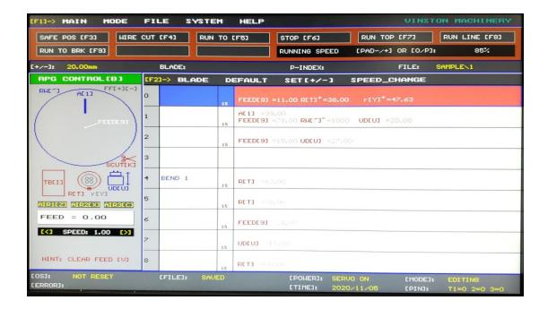
Using the three shortcut keys "Z", "X", "C" allows the user to manually turn the pneumatic cylinders on and off. Pressing each shortcut key once will change the current value from a 1 (Enabled) to a 0 (Disabled) or vise versa. This function is useful in the early stages of developing the program or to test the connections.
