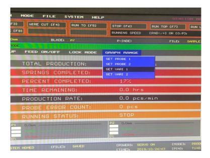
Press ENTER to bring up the selection window of the value for the variation tolerance of touch probe 1. The set value is 30%, meaning the feed viaration can be  $\pm$  40% of the default 10 mm feed.
