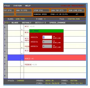
The pneumatic probe is enabled with a value of 1 and disabled with a value of 0. Whenever a pneumatic probe is enabled, it must be manually disabled within the program at a later point. It will not automatically retract after completing the designated task.
