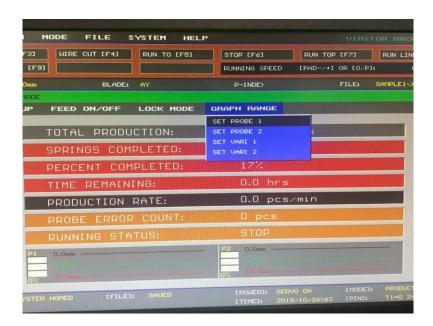
Press ENTER to bring up the selection window of the default feed\_value of probe #1. This value should be equal to or greater than the feed value in the probe designation.
