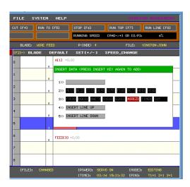
Select the AIR [Z] axis and press the Insert key.
