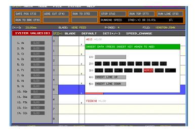
Select the item TIMER (V) option and press the INSERT key again. Highlight the TIMER component to bring up the follow option. The user can set a value from 0 to 5000, with each unit representing one millisecond. The maximum value is 5 (5000) seconds.
