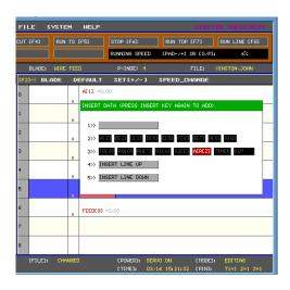
Select the AIR [Z] component and press the INSERT key. Set the AIR [Z] value back to 0 to retract the pneumatic probe.
