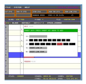
Highlight the AIR [Z] selection and press the INSERT key. With the Air [Z] component highlighted within the program line, press the ENTER key to configure the pneumatic probe:
