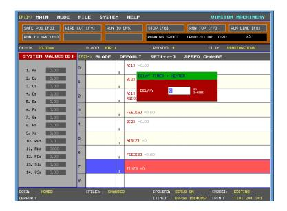
Press ENTER key to confirm changes. This feature is typically used to stabilize the spring as movements up to this point created unwanted vibrations.
